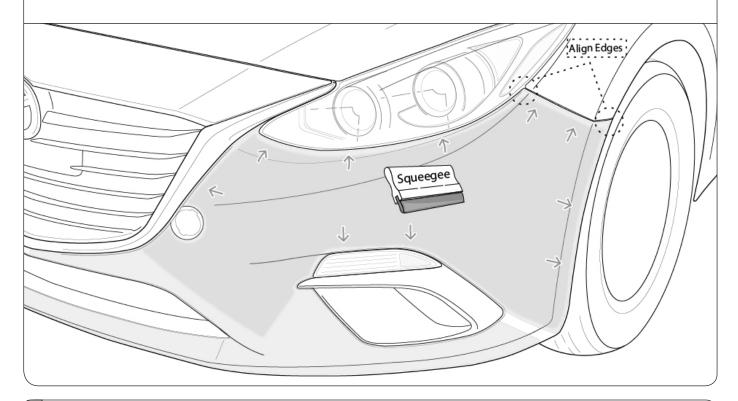
Squeegee around the bottom areas of the bumper and if necessary re-wet film.
